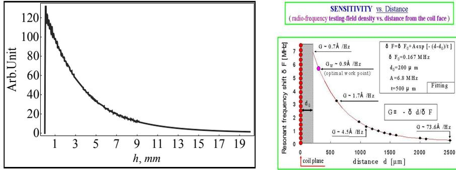
Fig. 1.  $H_x$  (or  $H_y$ , parallel to the coil face components) component vs. the distance ( $h$ ) from the coil surface, obtained from formula (13). The parameters of calculations are  $R \sin \theta = 5 \text{ mm}$ ,  $r = 0.05 \text{ mm}$ ,  $R_{\text{hole}} = 0.5 \text{ mm}$  and  $N = 100$  turns,  $R_{\text{coil}} = 10 \text{ mm}$ .
