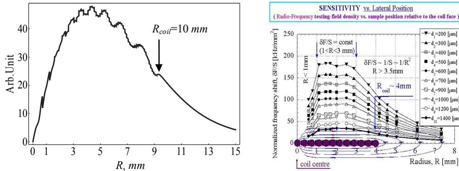
Fig. 2. The dependence of  $H_x$  (or  $H_y$ ) components on the distance  $R$  from the coil axis in the plane that is at  $5 \text{ mm}$  distance from the coil face, obtained from formula (13). The parameters of calculations are  $R \cos \theta = 5 \text{ mm}$ ,  $r = 0.05 \text{ mm}$ ,  $R_{\text{hole}} = 0.5 \text{ mm}$  and  $N = 100$  turns,  $R_{\text{coil}} = 10 \text{ mm}$ .
